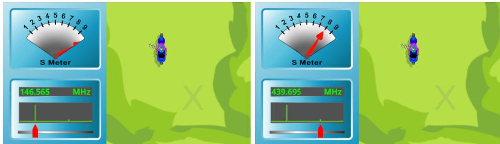
Figure 1.3: Switching to the third harmonic attenuates the signal.
